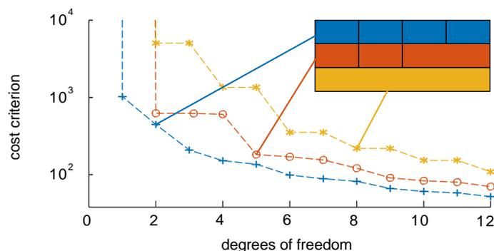
Fig.2 Performance criterion  $V^0$  (lower is better performance) as function of the number of feedforward filter parameters for the three different sampling sequences of Fig.1. Due to the additional control point, the non-equidistant sampling sequence (red) yields better performance than the conservative equidistant sampling sequence (orange).
