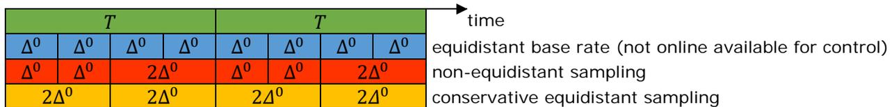
Fig.1 Example timeline of different processes executed on a single processor. Due to platform limitations, the equidistant base rate (blue) is not available for online control. The non-equidistant sampling (red) is available for control and provides an additional control point in each period (green) compared to conservative equidistant sampling (yellow).
