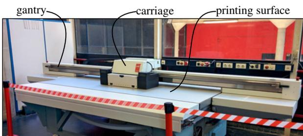
**Figure 1:** Océ Arizona 550 GT flatbed printer at the TU/e Motion Lab. The movements of the carriage and gantry introduce position dependence.
