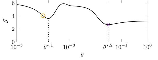
Fig. 4.  $\mathcal{J}$  for a grid in  $\theta$  and the corresponding optimal parameters. For  $\theta^{(0)} = 10^{-3}$ , the pre-existing approach (○) converges to the point near the local minimum, whereas the proposed approach (×) converges to the global minimum.
