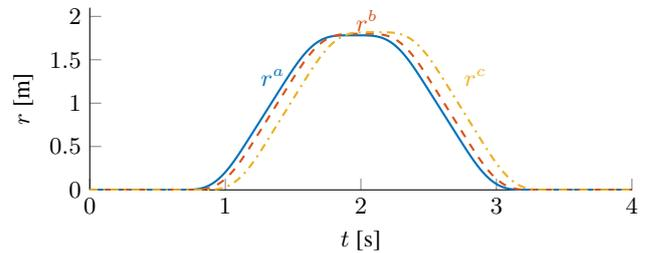
Fig. 7. A trial-varying reference signal is considered. Reference signal  $r^a$  (—) is active during trial  $j = 0, 1, 2$ ;  $r^b$  (---) during  $j = 3, 4, 5$ ; and  $r^c$  (-.-) during  $j = 6, 7, 8$ .
