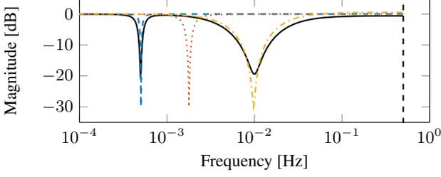
Fig. 3. The inverse system  $P^{-1}$  (—) and feedforward filters  $F(\theta = 10^{-5})$  (---),  $F(\theta = 10^{-3})$  (.....), and  $F(\theta = 10^{-1})$  (-.-). By design,  $F(\theta)$  is only able to (partially) compensate one of the resonances.
