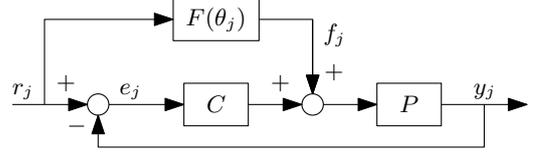
Fig. 2. Implementation of basis functions in  $f_j = F(\theta_j)r_j$ .
