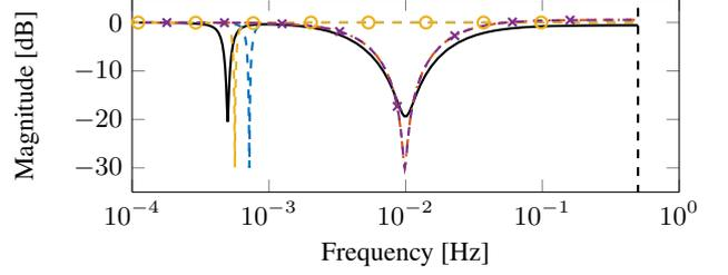
Fig. 5.  $F(\theta)$  for  $\theta^{*,1}$  (---),  $\theta^{*,2}$  (-.-), and pre-existing (· · ·) and proposed (· × ·) approach (both after ten iterations) partially compensate different resonances of  $P^{-1}$  (—).
