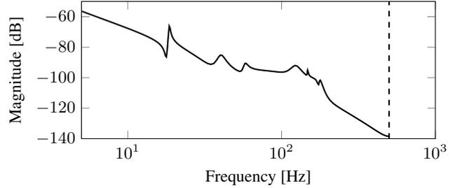
Fig. 6. Bode magnitude plot of the printer model.
