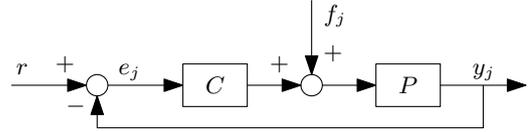
Fig. 1. Block diagram of closed-loop system under consideration.
