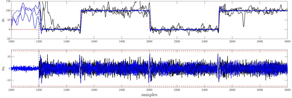
Fig. 2: Simulation results comparing the reference tracking performance of DeePC with averaging (black) and DeePC with IV (blue). For  $p = f = 20$  with  $\text{var}(e_k) = 0.1^2$  and  $\bar{N} = 500$ , the proposed IV method outperforms the original method in terms of the tracking error for three distinct realizations.
