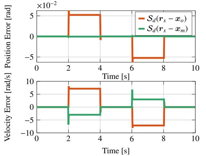
Fig. 7. Tracking error comparison of the 30th iteration. The dots are plotted for each 2 samples. The proposed state-tracking ILC using the non-causal state observer (—) is showing better on-sample state tracking results than previous method using only a causal state observer (—).
