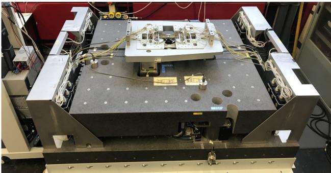
Fig. 6. Reticle stage setup at the motion lab of the TU/e.
