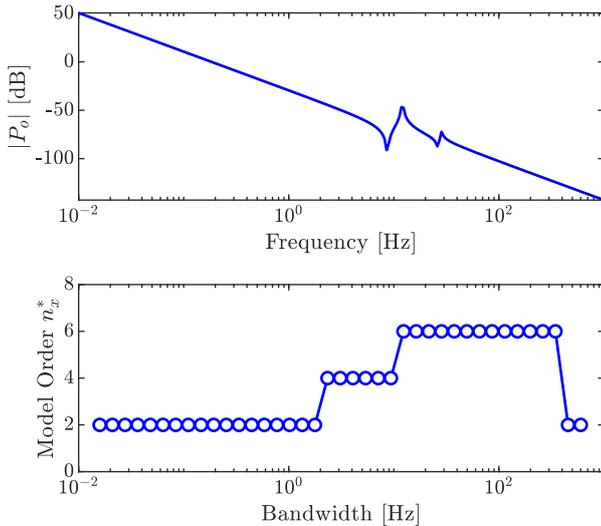
Fig. 5. Optimal model order as function of the desired bandwidth.
