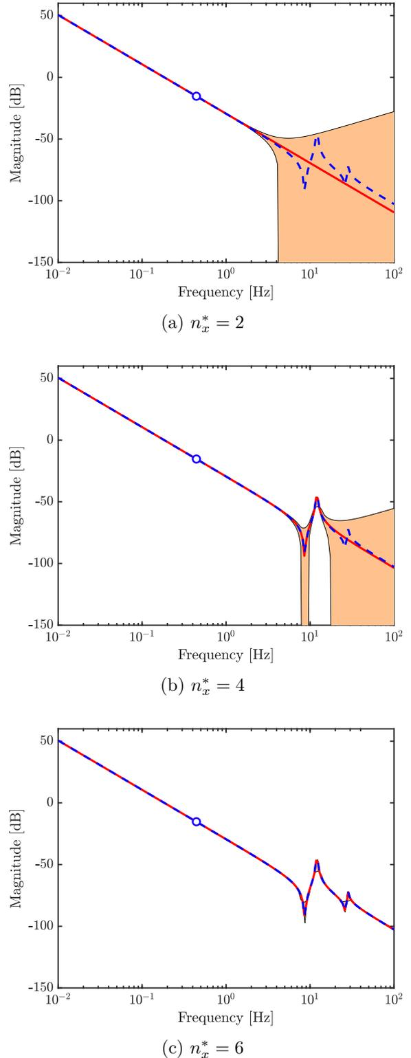
Fig. 3. Bode magnitude diagram of the nominal model  $\hat{P}$  (—), the true system  $P_o$  (---) and the robust-control-relevant model set  $\mathcal{P}^{RCR}$  (■). The desired bandwidth is indicated by (○).
