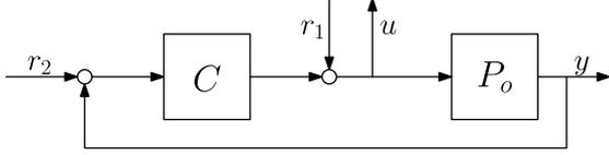
Fig. 1. Four-block feedback interconnection.
