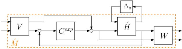
Fig. 2. Weighted closed-loop blockscheme.
