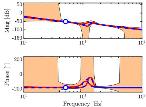
**Figure 1:** Multivariable Bode magnitude (top) and phase (bottom). True system  $P_o$  (—), nominal model  $\hat{P}$  (—), model set (■), and target bandwidth (○).
