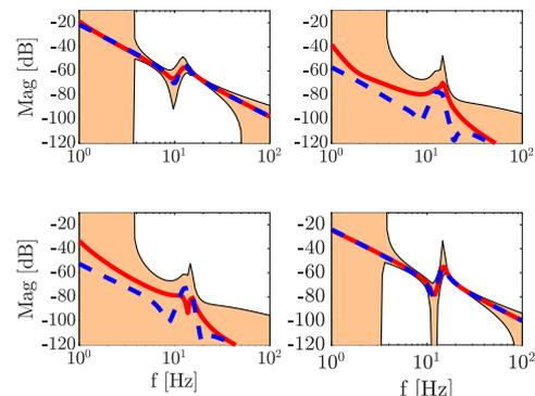
**Figure 2:** Element-wise Bode magnitude. True system  $P_o$  (—), nominal model  $\hat{P}$  (—), model set (■).
