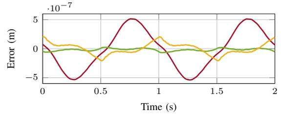
Fig. 10. Measured error of a piezoelectric actuator that aims to follow the reference trajectory (24). Three feedforward controllers are compared: 1) a linear feedforward controller (—) 2) a Prandtl-Ishlinskii based feedforward controller in yellow (—), 3) the feedforward controller developed in Section IV in green (—).
