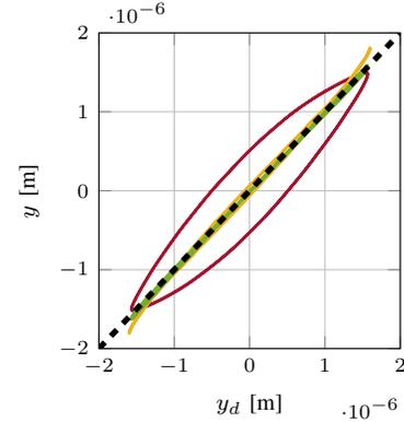
Fig. 11. Hysteresis loop from desired displacement to the measured displacement of a piezoelectric actuator. Three feedforward controllers are compared: 1) a linear feedforward controller (—) 2) a Prandtl-Ishlinskii based feedforward controller in yellow (—), 3) the feedforward controller developed in Section IV in green (—).
