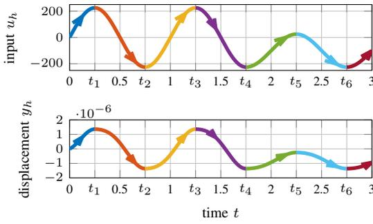
Fig. 1. Input  $u_h(t)$  given by (1) and corresponding output  $y_h(t)$ . Each color indicates one branch of the the hysteresis loop. The time instance of each branching point is indicated by  $t_i$ .
