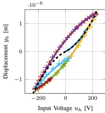
Fig. 8. Hysteresis loop when applying input signal (1). Each color indicates one branch of the the hysteresis loop. Experimental data from the piezoelectric actuator is given by crosses (+).
