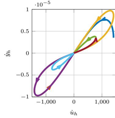
Fig. 3. Differential input-output pair of Example ?? when applying input signal (1). Each color indicates one branch of the hysteresis loop. The skeleton corresponding to this hysteric behaviour is given by the dashed black line (- -).
