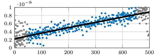
Fig. 7. Experimental data of the mapping  $M(p)$  in blue (●) and corresponding identified mapping exploiting Theorem 5 (—). The measurement points with a low signal-to-noise ratio which are not taken into account in the residual are indicated in gray (●).
