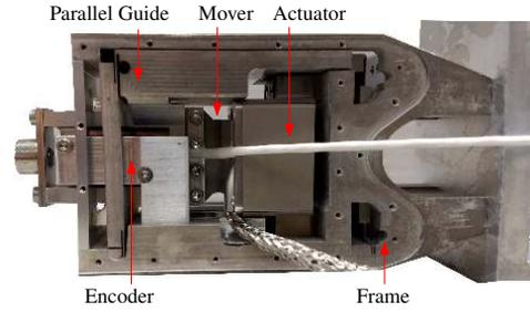
Fig. 6. Experimental setup with piezoelectric actuator.
