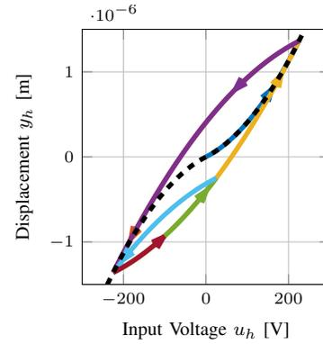
Fig. 2. Hysteresis loop when applying input signal (1). Each color indicates one branch of the the hysteresis loop. The skeleton corresponding to this hysteric behaviour is given by the dashed black line (- -). Experimental data from a piezoelectric actuator is given by crosses (+).
