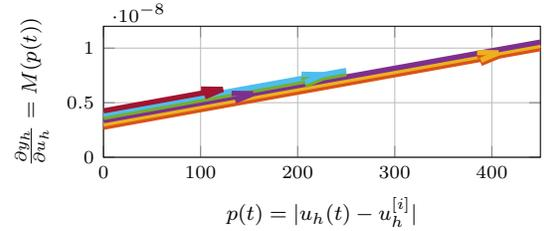
Fig. 4. The gradient  $\frac{\partial y_h}{\partial u_h} = M(p(t))$  with respect to  $p(t) = |u_h - u_h^{[i]}|$  corresponding to the hysteresis loop depicted in Fig. 2. To visualize the start and end point of each line all lines have a slight offset with respect to each other, in reality all lines perfectly overlap.
