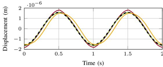
Fig. 9. Measured position of a piezoelectric actuator that aims to follow the reference trajectory depicted by the dashed line (- -). Three feedforward controllers are compared: 1) a linear feedforward controller (—) 2) a Prandtl-Ishlinskii based feedforward controller in yellow (—), 3) the feedforward controller developed in Section IV in green (—).
