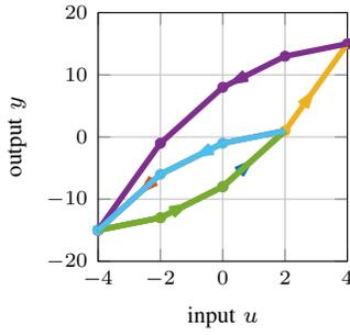
Fig. 6. Hysteresis loop of a Prandtl-Ishlinskii model with parameters as given in Example 2 with input signal as depicted in Fig. 4. Each color corresponds to a monotonic partition of the input signal as in Fig. 4. The dots (•) indicate the time instances where the input exceeds the threshold value of one of the play operators.
