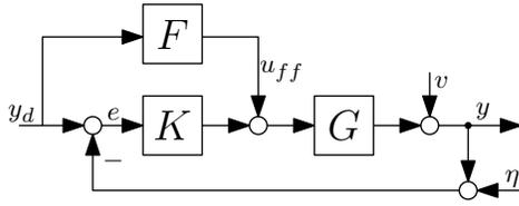
Fig. 1. Typical control architecture for servo control.
