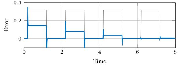
Fig. 2. Error signal, in blue (—), obtained from a closed-loop experiment as described in Procedure 1 with a scaled version of the desired trajectory depicted in gray (—). After each constant segment the value of  $c$  is increased leading to a  $e = 0$ , i.e., the correct value of  $c$  is found.
