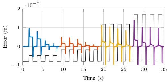
Fig. 7. Experimental validation of the tuning steps as introduced in Procedure 2 applied to a piezoelectric actuator. The desired trajectory (scaled and shifted in black (—)) is piecewise constant with 4 different amplitudes, each amplitude ensures an additional momentum  $p_j$  exceeds its threshold. The four tuning steps: decreasing  $w_1$  in blue (—); decreasing  $w_2$  in red (—); decreasing  $w_3$  in yellow (—); decreasing  $w_4$  in purple (—).
