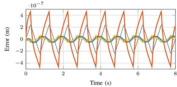
Fig. 8. Closed-loop experiment with piezoelectric actuator with a triangular desired trajectory (scaled and shifted in black (—)). Three different cases are studied: only feedback (—); with hysteresis compensation and corresponding identification procedure of 4 weights as in [9] (—); with feedforward compensation determined using the control-relevant identification procedure of four weights as described in Procedure 2 (—).
