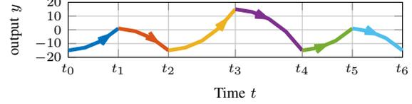
Fig. 5. Output  $y(t)$  of a Prandtl-Ishlinskii model with parameters as given in Example 2 with input signal as depicted in Fig. 4. Each color corresponds to a monotonic partition of the input signal as in Fig. 4
