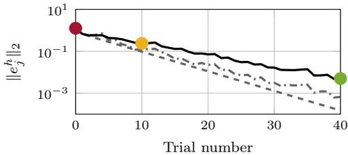
Fig. 8. Error norm  $\|e_j^h\|_2$  when applying an intermittent ILC controller designed following Theorem 4 (—), and Theorem 3 (---). The situation where all data is available at each trial  $j$  (---). The error norm  $\|e_j^h\|_2$  of trails  $j \in \{0, 10, 40\}$  as depicted in Fig. 7 are highlighted with their corresponding color.
