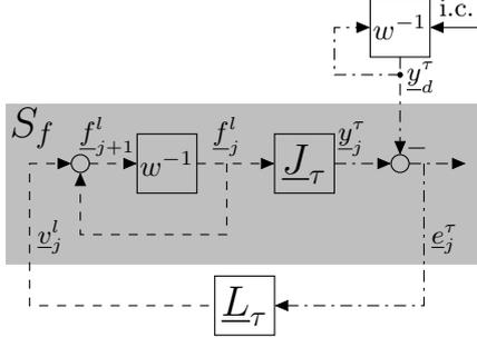
Fig. 5. ILC setup with state  $f_j^l$ .
