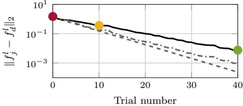
Fig. 9. Input difference norm  $\|f_j^l - f_d^l\|_2$  when applying an intermittent ILC controller designed following Theorem 4 (—), and Theorem 3 (---). The situation where all data is available at each trial  $j$  (---). The norm  $\|f_j^l - f_d^l\|_2$  of trails  $j \in \{0, 10, 40\}$  as depicted in Fig. 7 are highlighted with their corresponding color.
