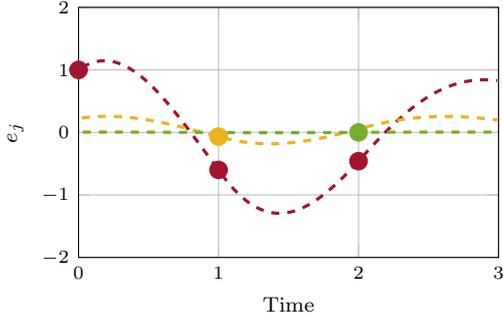
Fig. 7. Error  $e_j$  at trial  $j = 0$  (---),  $j = 10$  (---), and  $j = 40$  (---) when applying an intermittent ILC controller of Theorem 4 with the available error at the time-stamps,  $e_j^\tau$  indicated by dots (●).
