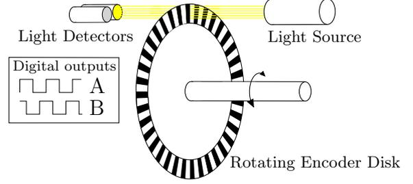
Fig. 3. Schematic representation of incremental encoder
