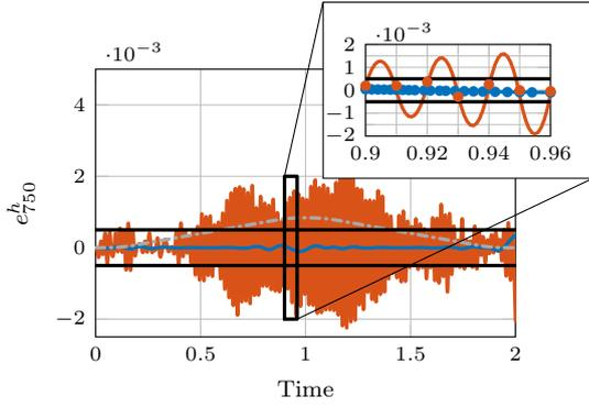
Fig. 10. Error  $e_{750}^h$  at trial 750 after applying traditional ILC with quantized data (—) and after applying intermittent ILC controller of Theorem 4 with exact data at the time-stamps (—). In the zoom the time-instances of the available error data are indicated by dots (• and •). The quantization level is indicated by (—). The dash-dotted line (---) depicts the reference scaled down by a factor 400.
