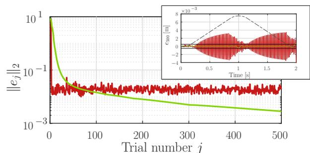
**Figure 1:** Error norm  $\|e_j^h\|_2$  when applying traditional quantized ILC (—) and when applying the decentralized ILC controller (—). Error  $e_{500}$  at trial 500 after applying traditional quantized ILC (—) and after applying the decentralized ILC controller (—).
