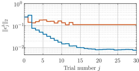
(b) Error norm  $\|e_j^h\|_2$  when applying traditional quantized ILC (—) and the time-stamped ILC of Section III (—).
