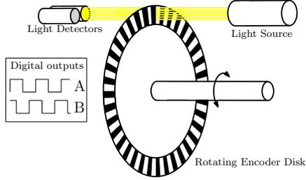
Fig. 1: Schematic representation of incremental encoder
