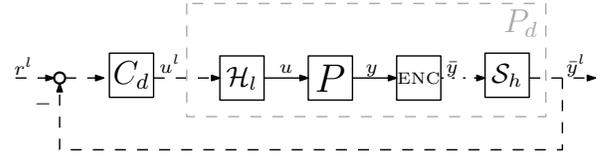
Fig. 3: Block scheme of feedback control scheme with incremental encoder.
