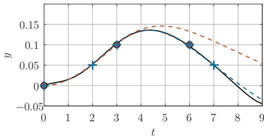
(c) Reference  $r$  (—) and the position of mass-spring-damper system during the 30-th trial when applying traditional quantized ILC (---) and time-stamped ILC of Section III(---). The equidistant data points used by quantized ILC are indicated by red marked dots(●); the data points used in time-stamped ILC are indicated by blue crosses (+).
