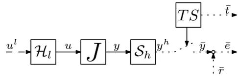
Fig. 4: Multirate time-stamped ILC setup
