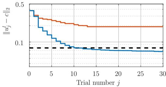
(a) Norm  $\|u_j^l - u_\infty^l\|_2$  when applying traditional quantized ILC (—) and norm  $\|u_j^l - c\|_2$  when applying time-stamped ILC of Section III (—). The edge of the sub-optimal 2-norm ball  $\mathcal{B}_p(c, d)$  is indicated by the dashed black line (—)
