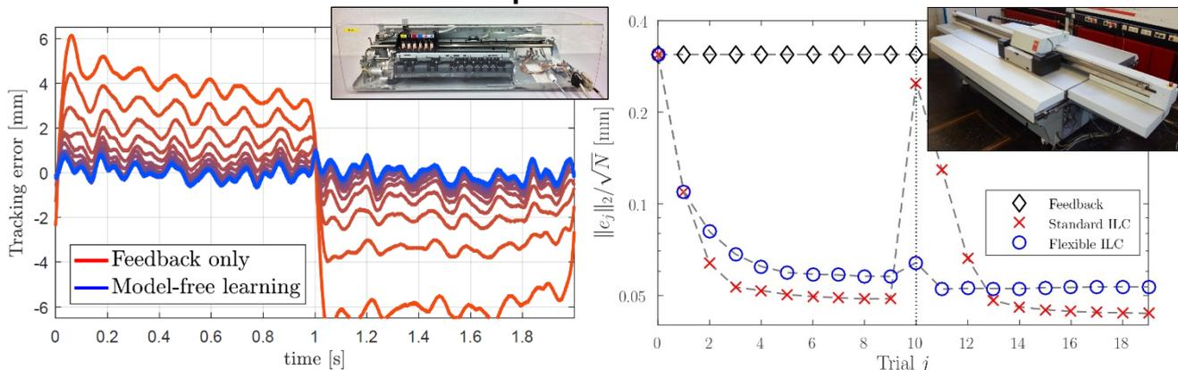
**Figure 1:** Experimental results using learning control: high performance can be achieved without using models (left), and robustness to non-repeating disturbances (in trial 10) is obtained using flexible ILC. (right).
