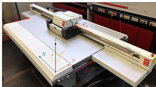
**Figure 1:** The carriage of the Arizona flatbed printer is controlled in its planar coordinates  $y$ ,  $x$  and  $\phi$ , by using the actuator forces  $F_y$ ,  $F_l$  and  $F_r$ .
