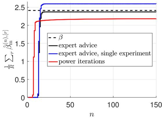
Fig. 5. Data-driven  $\mathcal{H}_\infty$ -norm estimate: a comparison.
