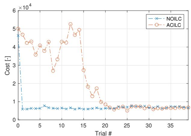
**Figure 1:** Cost per trial for model-based NOILC with basis functions and model-free ACILC experiments.
