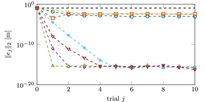
(b) For the approximate inverse techniques NPZ-Ignore (—), ZPETC (—), and ZMETC (—) convergence is enforced through a robustness filter  $W = Q^*Q$  at the cost of performance  $\|e_j\|_2$ . All other techniques, i.e., stable inversion (—), norm-optimal feedforward (—),  $\mathcal{H}_\infty$  preview control (—), and  $\mathcal{H}_2$  preview control (—), converge to zero error up to numerical precision. Norm-optimal ILC is exact and therefore converges in a single trial.
