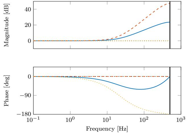
**Fig. 5.**  $HF$  for NPZ-Ignore (—), ZPETC (---), and ZMETC (⋯).  $HF$  has zero phase for ZPETC and zero magnitude for ZMETC.
