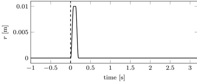
**Fig. 4.** Reference trajectory  $r$  consists of a forward and backward movement and includes pre-actuation and post-actuation time.
