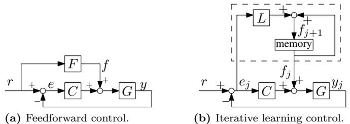
**Fig. 1.** The feedforward (a) and ILC (b) design problem are equivalent to finding  $u$  in (c) that minimizes  $e$ .
