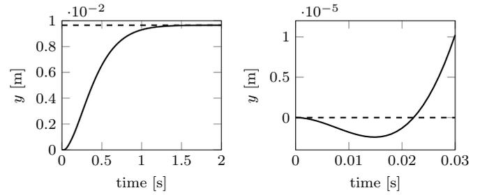
**(a)** Response to positive step. **(b)** Initially, the system moves in negative direction.
