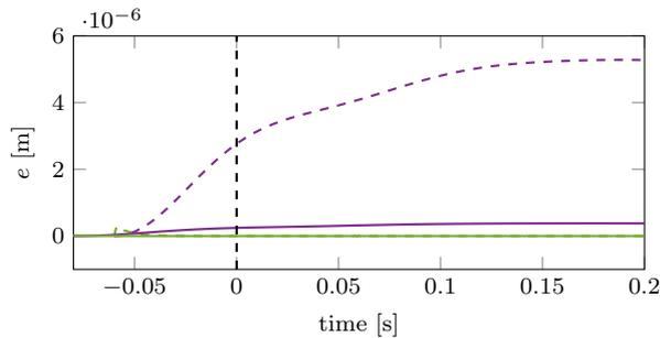
(b) The infinite design of stable inversion (---), (—) introduces significant boundary errors on a finite interval, whereas these are much smaller for the finite time design of norm-optimal feedforward (---), (—).
