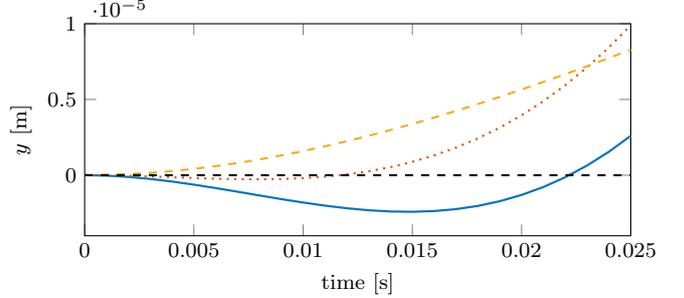
(c) The step responses of the transfers  $u_1 \rightarrow y$  (—) and  $u_2 \rightarrow y$  (····) initially move in opposite direction of the final value, confirming nonminimum-phase behavior. The step response of the down-squared system (---) moves in the direction of the final value, confirming minimum-phase behavior.
