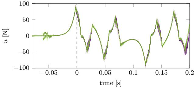
(a) Norm-optimal feedforward, (---), (—) generates a non-zero input  $u$  at the begin of the task to compensate for boundary effects. The effect is larger for 60 samples preview (---) than for 80 samples preview (—). Stable inversion generates identical  $u$  with 60 samples preview (---) and 80 samples preview (—) for  $t \geq -0.06$ , whereas for 80 samples preview  $u$  is non-zero for  $-0.08 \leq t < -0.06$ .
