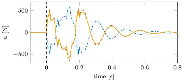
**Fig. 13.** For the two-input, single-output system of Fig. 12, the transformation (9) enables the use of exact and direct inversion (1) yielding bounded inputs  $u_1$  (---),  $u_2$  (---), and combined input  $u$  (—).
