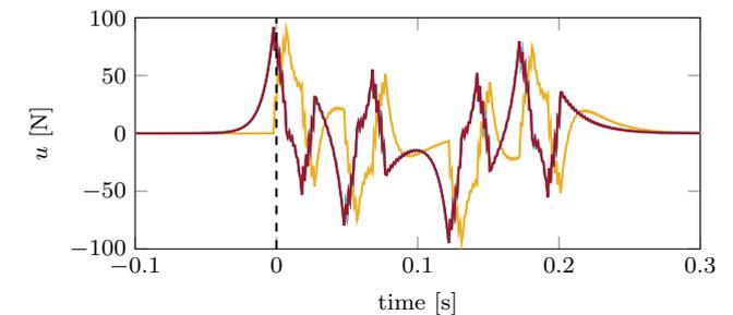
(b) ZMETC (—), stable inversion (—), norm-optimal feedforward (—),  $\mathcal{H}_\infty$  preview control (—), and  $\mathcal{H}_2$  preview control (—).**Fig. 9.** Command signal  $u$ . The signals in (a) are unacceptably large. The signals in (b) are satisfactory.
