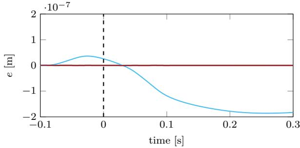
(b) Stable inversion (—), norm-optimal feedforward (—),  $\mathcal{H}_\infty$  preview control (—), and  $\mathcal{H}_2$  preview control (—). Norm-optimal, stable inversion, and  $\mathcal{H}_2$  preview are overlapping.
