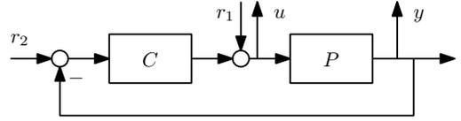
Fig. 1. Feedback configuration.
