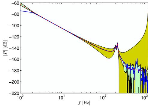
Fig. 5. Bode magnitude diagram of transfer function estimate of  $P_o$  (solid), model  $\hat{P}$  (dashed), plant set  $\mathcal{P}$  using nonparametric bound  $\gamma(\omega_i)$  (cyan), plant set  $\mathcal{P}$  using static overbound (yellow).
