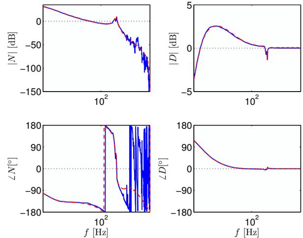
Fig. 3. Bode diagram of identified  $N_o, D_o$  (solid) and estimated  $\hat{N}, \hat{D}$  (dashed).
