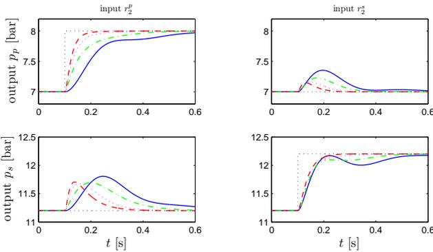
Fig. 4. Closed-loop step responses ( $r_2 \mapsto y$ ): initial controller  $C^{\text{exp}}$  (solid blue), optimal robust controller  $C^{\text{RCR}}$  (dashed red),  $C^{\text{ADD}}$  (dash-dotted green), and  $C^{\text{DY}}$  (dotted).
