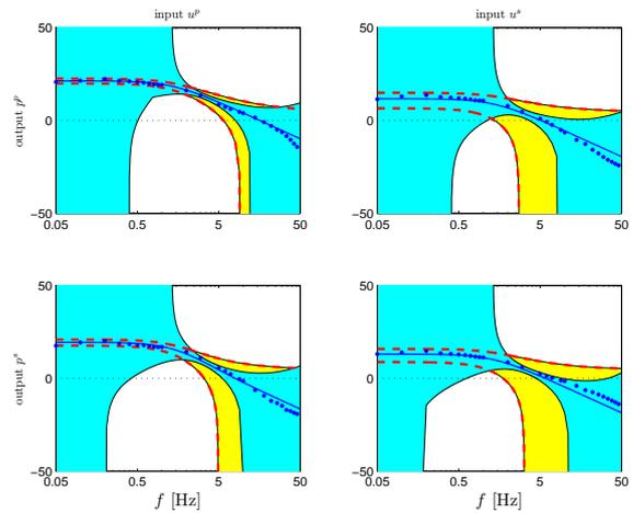
Fig. 3. Nominal model  $\hat{P}$  (solid blue), frequency response function estimate  $\tilde{P}_o(\omega_i), \omega_i \in \Omega^{\text{id}}$  (blue dots), and model set  $\mathcal{P}^{\text{RCR}}$  (cyan) and  $\mathcal{P}^{\text{ADD}}$  (yellow, red dashed).
