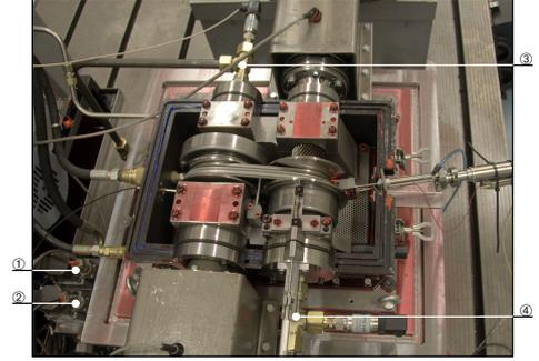
Fig. 2. Photograph of the experimental CVT system, where ①: primary servo valve  $V_p$ , ②: secondary servo valve  $V_s$ , ③: pressure measurement  $p_p$  at primary hydraulic cylinder, ④: pressure measurement  $p_s$  at secondary hydraulic cylinder.
