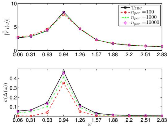
Fig. 5. Results of model validation test for varying  $n_{\text{per}}$ . Estimated deterministic disturbance model (top), estimated model uncertainty (bottom).
