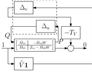
Fig. 4. Recasting Figure 3 as an implicit LFT.
