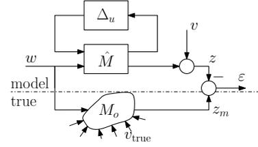
Fig. 1. Model validation setup.
