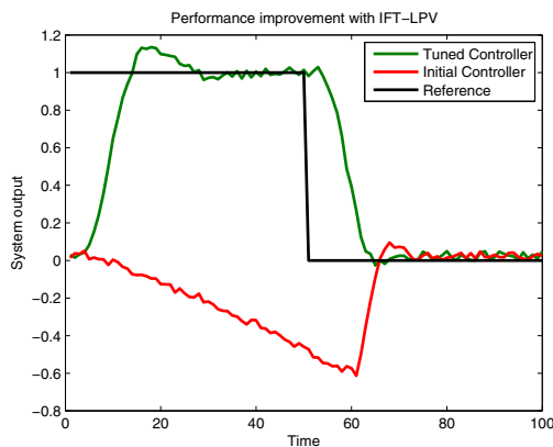
Fig. 3. Comparison of controller performance before and after data-based controller tuning with IFT.
