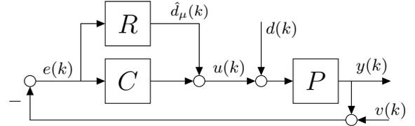
Fig. 1. Control setting with multi-period disturbance  $d(k)$  with  $k \in \mathbb{N}$  and repetitive controller  $R$ .
