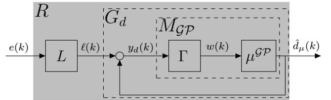
Fig. 3. Gaussian process repetitive controller  $R$  with Gaussian-process-based buffer  $M_{GP} = \mu^{GP}\Gamma$  and internal model of the disturbance generating system  $G_d$ .
