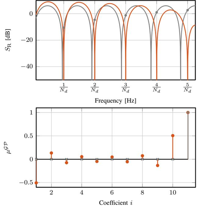
Fig. 7. Example 1: Modifying sensitivity function  $S_R$  (top plot) and impulse response of  $M_{\mathcal{GP}}$  (bottom plot) for GPRC without smoothness and  $T = 11$  (—), and with smoothness with  $T = 10.5$  (—). Including smoothness yield that many FIR coefficients  $\mu^{\mathcal{GP}}$  are non-zero (●) for automatic interpolation, which enables suppression at  $1/N_d$  and higher harmonics, whereas traditional RC performance in much worse (×).
