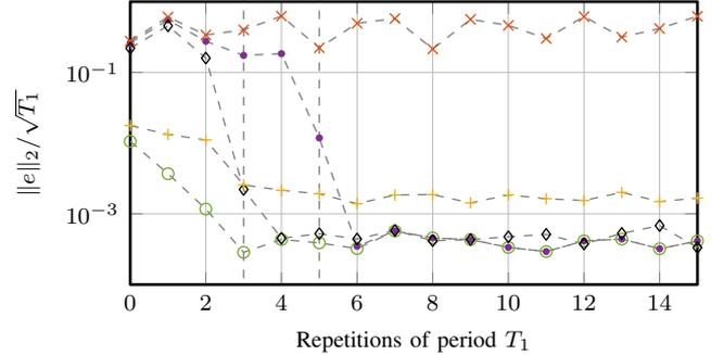
Fig. 14. Error 2-norm as function of  $T_1$  with PD ( $\times$ ). GPRC with  $N_1 = 52$  in ( $\diamond$ ) that converges after  $3T_1$ , and with buffer size  $N_1 = 104$  ( $\bullet$ ) GPRC converges after  $5T_1$ . With a time-varying prior noise variance (41) the error ( $\circ$ ) convergence is much faster ( $l = 1$ ), converges to a larger error with a larger smoothness ( $l = 3$ ) ( $+$ ).
