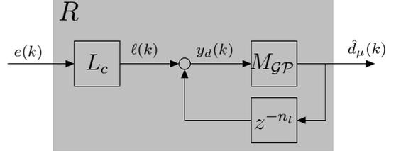
Fig. 5. Practical RC implementation with a non-causal learning filter  $L$  with causal equivalent  $L_c$  and preview  $z^{n_l}$ .
