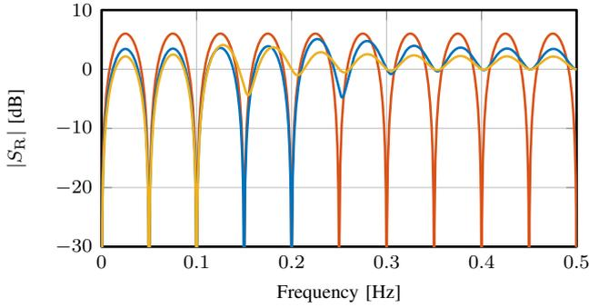
Fig. 9. Modifying sensitivity with GPRC for a periodic kernel with three different levels of smoothness  $l = 10^{-6}$  (—),  $l = 10$  (—) and  $l = 100$  (—), showing that smoothness improves robustness for noise and reduces disturbance rejection at higher frequencies.
