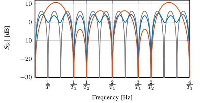
Fig. 10. Modifying sensitivity  $S_R$  for multi-period GPRC with  $n_d = 2$ ,  $T_1 = 20$  and  $T_2 = 15$  samples with buffer size  $N_1 = T_1 + T_2 = 35$  samples (—) and  $N_2 = \text{lcm}(T_1, T_2) = 60$  samples. As a comparison, the traditional RC with  $N = 60$  is also shown (—).
