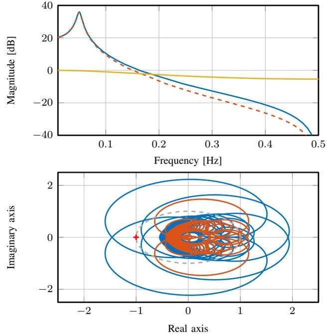
Fig. 16. Top plot shows the true system  $P$  (—), a perturbed model (—) that is used for RC as well as the model mismatch (—) that is significant (up to  $> 100\%$ ) beyond 0.1 Hz. The bottom plot shows the Nyquist stability test for smoothness  $l_1 = l_2 = 10$  (—) that is unstable, by increasing the smoothness to  $l_1 = 50$  and  $l_2 = 10$  the RC is stabilized (—) since there are no encirclements of the point  $-1 + 0i$ .
