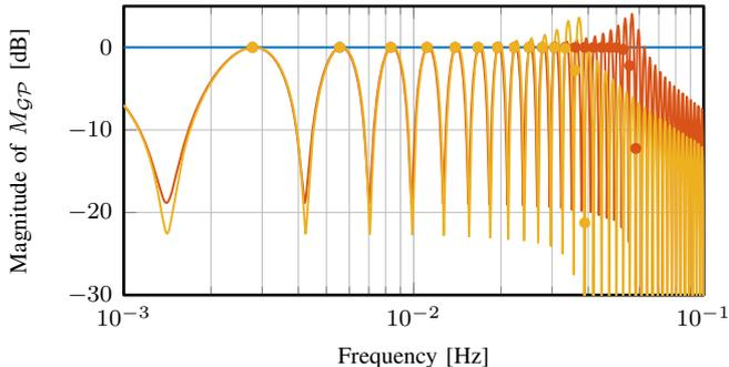
Fig. 12. Magnitude of  $M_{GP}$  for a periodic kernel with  $n_d = 1$  and  $T = 360$  and three settings of smoothness, i.e.,  $l = 10^{-3}$  (—),  $l = 0.5$  (—) and  $l = 1$  (—). The markers (●) and (●) indicate fundamental frequencies  $f = \frac{1}{T}$  and harmonics (top plot). This shows that smoothness leads to a low-pass characteristic in  $M_{GP}$ , which in turn increases robustness.
