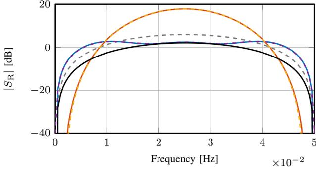
Fig. 8. Modifying sensitivity  $S_R$  with traditional RC (---) as baseline. HARC in [28] for noise robustness (---) with  $N = 3T$  is recovered by GPRC a periodic kernel (—). Also HARC for period variations (---) is recovered with a locally periodic kernel (—). Introducing smoothness (—) outperforms noise-robust HARC with a smaller buffer size  $N = T$ .
