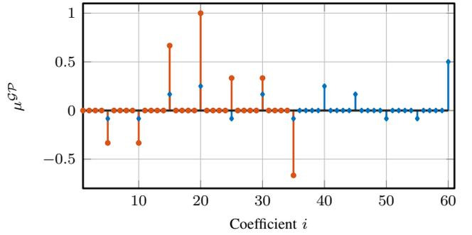
Fig. 11. FIR coefficients  $\mu^{\mathcal{GP}}$  with a multi-period kernel where  $n_d = 2$ ,  $T_1 = 20$ ,  $T_2 = 15$ , yielding non-zero FIR coefficients  $\mu^{\mathcal{GP}}$  at  $T_1$ ,  $T_2$  and the difference between them for  $N_1 = 35$  (○) and with  $N_2 = 60$  (◇).
