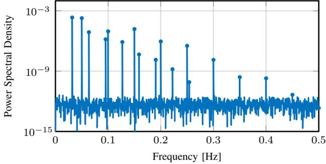
Fig. 13. Power spectral density of the multi-period disturbance, containing two fundamental periods  $T_1 = 20$  samples and  $T_2 = 31.5$  samples.
