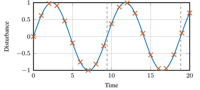
Fig. 2. Example: a continuous time disturbance  $d^c(t)$  (—) with period  $T = 3\pi$  from which discrete samples  $d(k)$  (×) with sample frequency 1 Hz are taken, i.e., the discrete time sequence  $d(k)$  is non-periodic for all  $k$  while the continuous time signal  $d^c(t)$  is periodic with the period time  $T \in \mathbb{R}$ .
