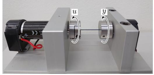
Fig. 5. Experimental setup of a two-inertia system connected via a flexible shaft. The motor on the left side is used as an input  $u$  and the encoder on the right side is used as an output  $y$ , respectively.
