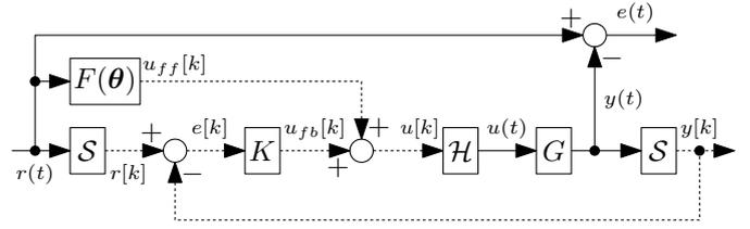
Fig. 1. Tracking control diagram. The continuous-time system  $G$  is controlled by the feedforward controller  $F(\theta)$  and the discrete-time feedback controller  $K$  with sampler  $\mathcal{S}$  and zero-order-hold  $\mathcal{H}$ . The objective is to minimize the continuous-time error  $e(t)$ . The solid and dotted lines denote the continuous-time and discrete-time signals, respectively.
