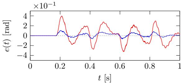
Fig. 8. Tracking error  $e(t)$  in experiment with  $\Psi = [\dot{r}, \Psi_a, \Psi_s]$ : using backward differentiator (—) and multirate zero-order-hold differentiator (—). The feedforward using the multirate zero-order-hold differentiator outperforms that using the backward differentiator in both rigid and flexible modes.
