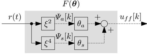
Fig. 2. Linearly parameterized feedforward with acceleration and snap.
