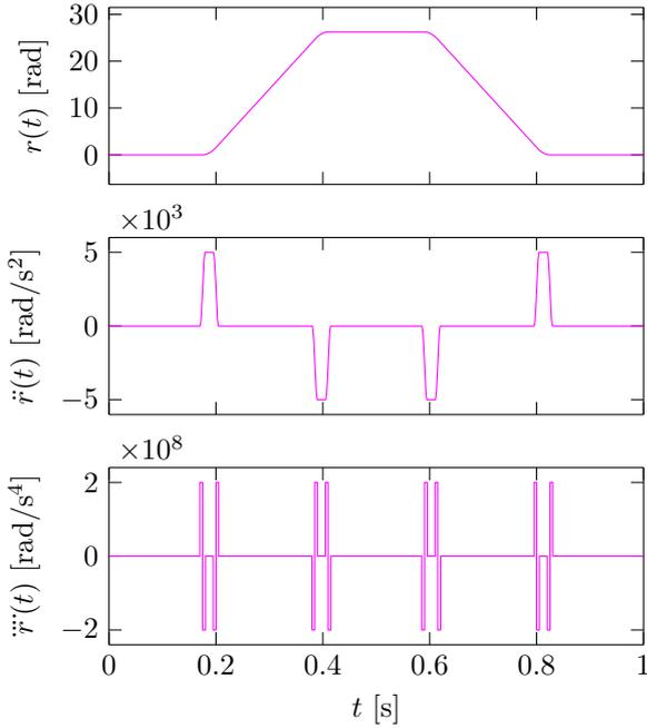
Fig. 7. Continuous-time 4<sup>th</sup> order polynomial trajectory reference: position  $r(t)$ , acceleration  $\ddot{r}(t)$ , and snap  $\dddot{r}(t)$ .
