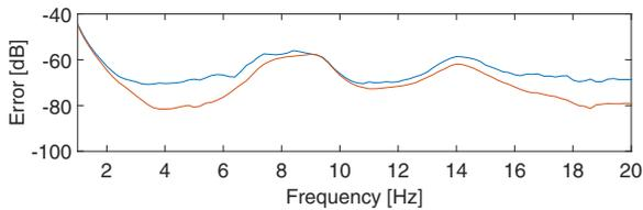
Fig. 4: Comparison between the simulation errors of the LRM for each LTI measurement (blue) and using the 2D approach (red). The errors are the root mean square errors over the scheduling parameters.
