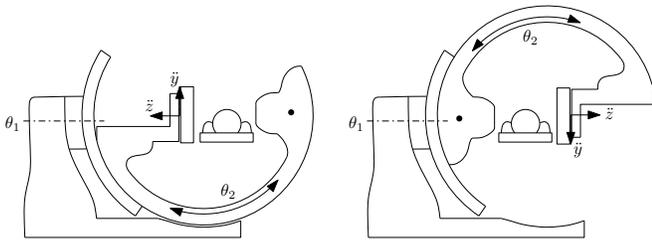
Fig. 3: Schematic representation of the Philips Allura Centron in two positions of the roll-rotations, i.e.,  $\theta_2 = -90$  and  $\theta_2 = 90$  degrees.
