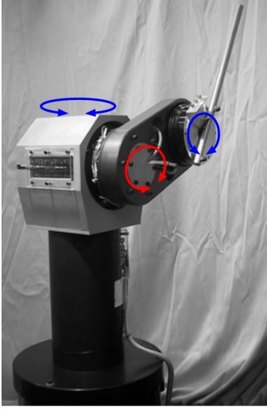
Fig. 4. RRR Robot - 3 rotational DOF robot present at the Department of Mechanical Engineering of the Technische Universiteit Eindhoven. Only the red rotational DOF is considered in this work. Picture from Kostić (2004).
