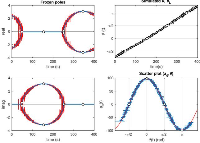
Fig. 3. Identification results on a simulation example. Left: Evolution of frozen poles (top: real part, bottom: imaginary part) (blue: estimated; red: true, locally linearised around  $\theta(t)$ ). Top right: Simulated  $\theta(t)$  (black) and trend  $\theta_L(t)$ . Bottom right: blue:  $(\hat{a}_0(t), \theta(t))$ , red:  $mg \cos(\theta)$ . The black circles indicate corresponding points of interest in the four plots.
