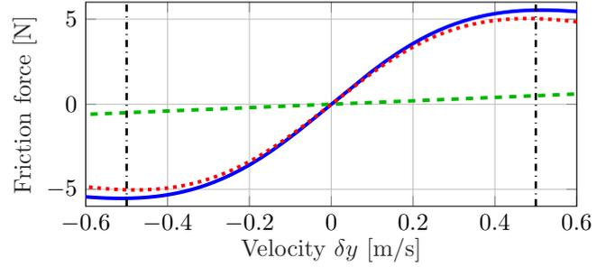
Fig. 3. Stribeck-like friction curve (—) of example system (21) with  $c_1 = 1$ ,  $c_2 = 20$ ,  $\alpha = 2.5$ , consisting of a linear (---) and nonlinear contribution (····). This nonlinearity can be approximated up to arbitrary accuracy by  $\mathcal{F}_\varphi$  on the domain covered by  $r$  (---).
