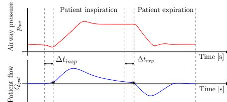
**Figure 1:** Typical pressure supported patient breath, where the ventilator supports the patient inspiration after  $\Delta t_{insp}$  seconds and cycles off  $\Delta t_{exp}$  seconds after the patient's expiration.
