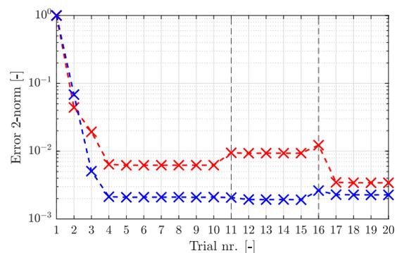
**Figure 1:** Comparison of the error 2-norm per trial for linear parametrized feedforward (-) and the proposed method (-). In order to show the flexibility of the methods, the motion task is changed at trials 11 and 16. This task change is indicated by vertical dashed lines.
