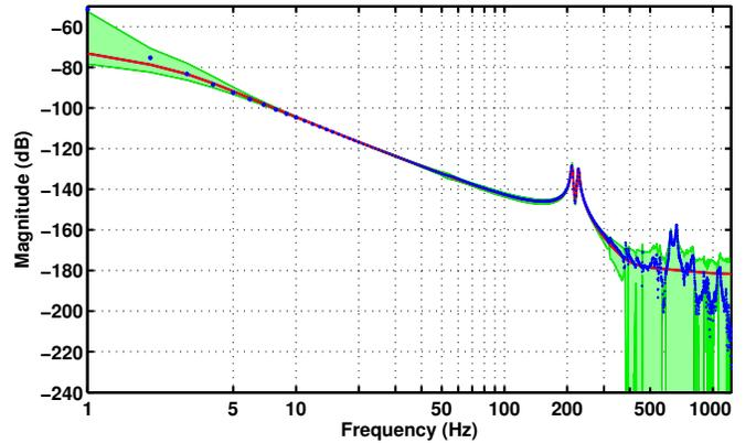
Fig. 6. Bode magnitude plot of the identified transfer function estimate of  $P_o$  (dotted), the constructed 7th order coprime factor model  $\hat{P}$  (solid), and the candidate plant set  $\mathcal{P}_{dY}(C)$  obtained through model validation (green).
