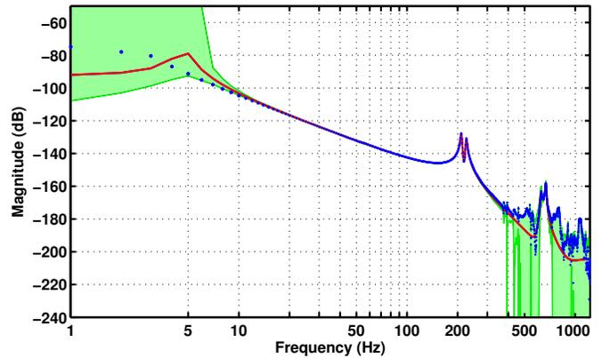
Fig. 10. Identified plant set based on a 11th order model  $\hat{P}$ .
