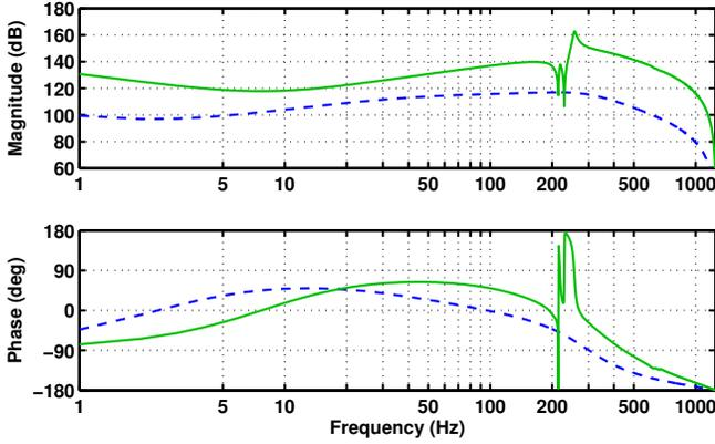
Fig. 5. Initial controller, designed with standard loop-shaping techniques (dashed), and robust controller, synthesized based on the 7th order plant set (solid).
