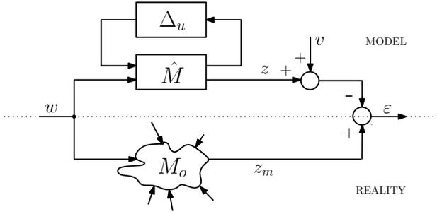
Fig. 3. Model validation setup.
