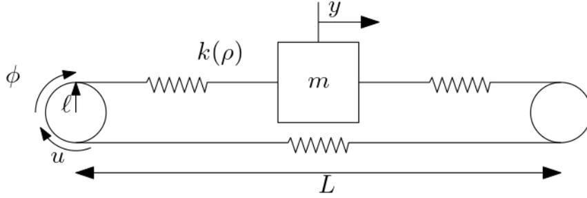
Figure 2: Timing-belt pulley system considered, with position-dependent spring stiffness  $k(\rho)$ .
