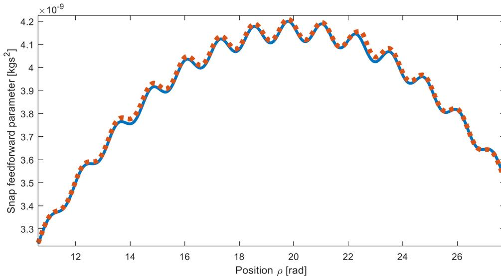
Figure 3: Learned (dotted orange) and true (solid blue) position-dependent snap feedforward parameter of the pulley system.
