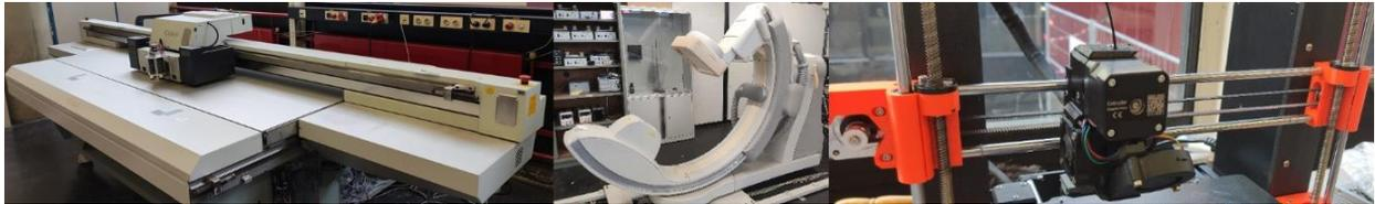
Figure 1: Example position-dependent systems. Left: position-dependent flatbed printer. Center: position-dependent image guided therapy system. Right: timing-belt pulley system with position-dependent stiffness.
