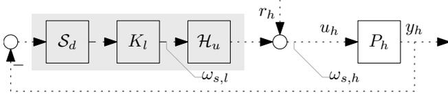
Fig. 1. Multirate feedback structure for system identification considered in this paper, with downsampler  $S_d$ , low-rate controller  $K_l$ , a multirate zero-order-hold reconstructor  $\mathcal{H}_u$  and high-rate plant  $P_h$ .
