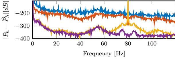
Fig. 4. Modeling error  $|P_h - \widehat{P}_h|$  for ETFE (—), LPM (—), Time-lifted (—) and frequency-lifted (—).
