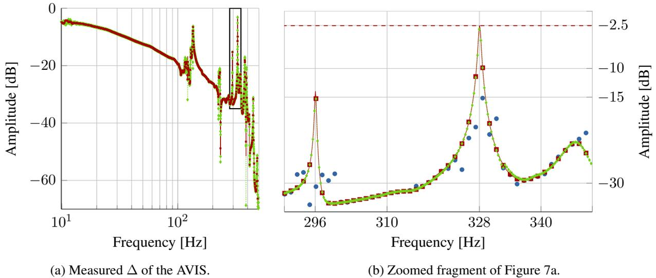
Figure 7: Measured  $\Delta$  of the AVIS. The FRF estimated by the LPM ( $\bullet$ ) and LRM ( $\blacksquare$ ) on a sparse frequency grid is shown. It can be observed that the LPM (4, 2, 2) is unable to properly capture the resonance peaks. By interpolating the LRM ( $- \blacksquare -$ ) the estimate of the peak amplitude near 329 Hz is improved by 7.5 dB. Both the interpolation and the peak estimate are validated against a four times denser data record ( $\cdots \bullet \cdots$ ).
