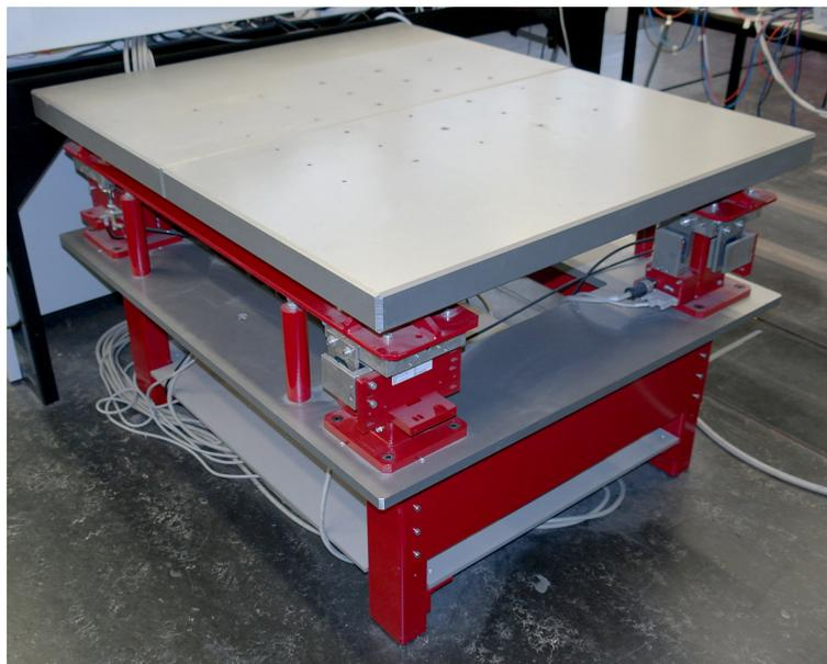
Figure 4: The active vibration isolation system (AVIS).
