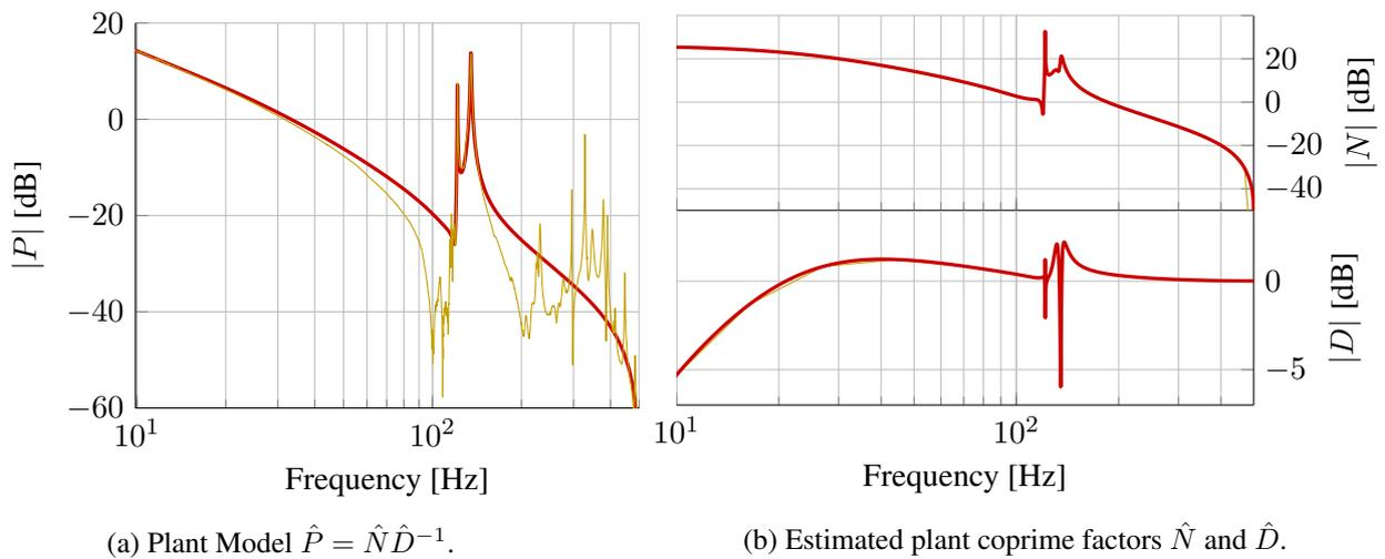
Figure 6: Estimated parametric model  $\hat{P} = \hat{N}\hat{D}^{-1}$  (—■) of the AVIS and a measured FRF (⋯♦).
