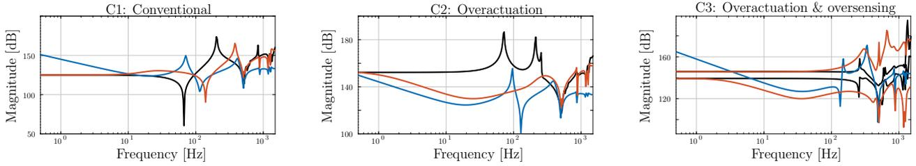
Fig. 5. Singular values of the different controllers for cases C1-C3. In all cases, the  $\mathcal{H}_\infty$ -optimal controllers  $\bar{K}_y$  (red) better approximate the MSCs  $\bar{K}_y^{\text{ms}}$  (black), than the traditional controllers  $\bar{K}_y^{\text{trad}}$  (blue).
