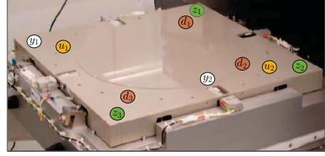
Fig. 2. Experimental setup: prototype wafer stage.
