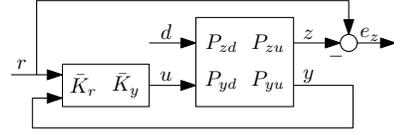
Fig. 1. General two-DOF controller structure in inferential control setup.
