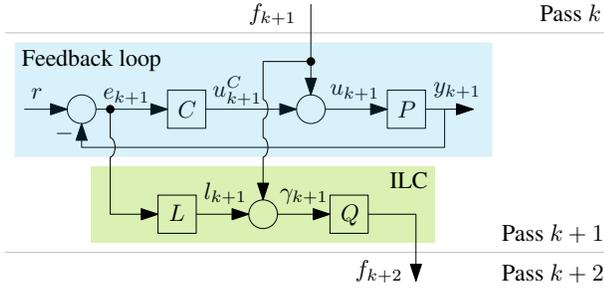
Fig. 1: Standard ILC with feedback control in a parallel configuration.
