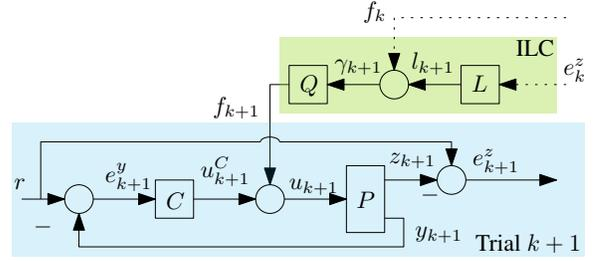
Fig. 2: Parallel inferential ILC structure, with 1-DOF feedback controller.
