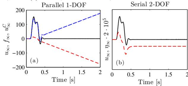
Fig. 5: Left (a), converged command signals  $u_\infty(p)$  (black solid),  $f_\infty(p)$  (dashed red), and  $u_\infty^C(p)$  (dashed-dotted blue). The parallel inferential ILC structure is not stable along the pass: the command signals of the feedback controller and the ILC grow unbounded with opposite sign, see Theorem 5, due to the interplay of  $C(z)$  with the ILC.
