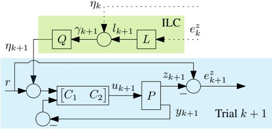
Fig. 3: Serial inferential ILC structure, with 2-DOF feedback controller.
