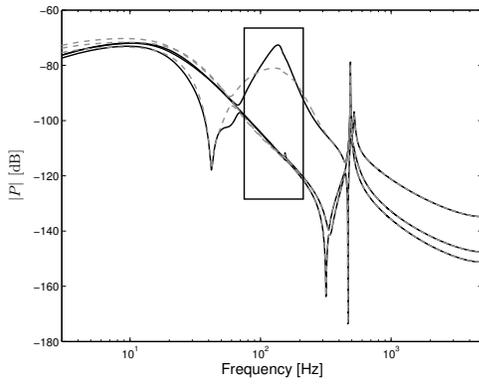
Fig. 10. The singular values of the process sensitivity  $SP$  for classical weighting (black) and multivariable weighting functions (dashed gray) show that a significant reduction is obtained in  $[40, 200]$  [Hz] as a result of multivariable weighting functions.
