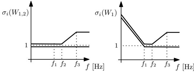
Fig. 4. Weighting  $W_{1,2}$  and multivariable weighting function  $W_1$ .
