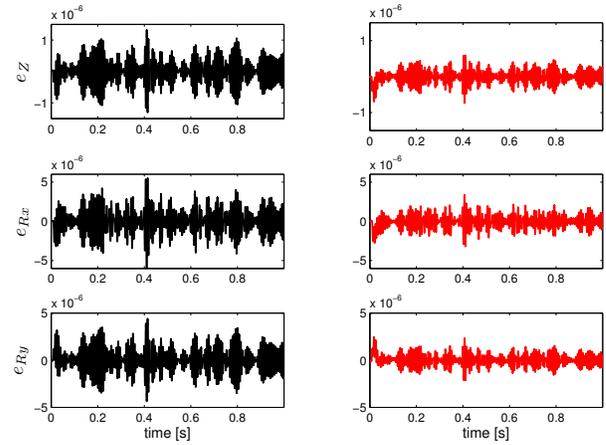
Fig. 11. Measured time domain responses for  $C^{class}$  (left) and  $C^{mimo}$  (right) show a reduction of approximately 50 [%] in the peak value of the error signal  $e$  due to  $C^{mimo}$ .
