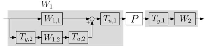
Fig. 5. Multivariable weighting function design.
