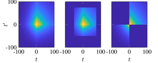
Fig. 3. Examples of modified non-causal stable spline kernels (8): full non-causal (left); truncated for finite preview and delay (middle); zero correlation between causal ( $t, t' \geq 0$ ) and anti-causal ( $t, t' < 0$ ) elements (right).
