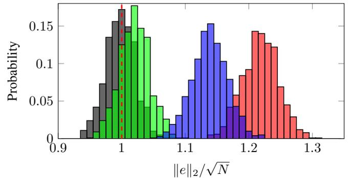
Fig. 5. Monte Carlo simulations: feedforward performance  $\|e\|_2$  with estimated non-causal inverse models. The developed non-causal kernel-based approach (■) closely approaches the perfect inverse-model feedforward  $P^{-1}$  (■), whereas using only a causal kernel (■) or none at all (■) leads to deteriorated performance. The noise variance  $\sigma_y^2$  is indicated by ---.
