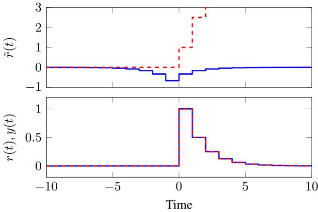
Fig. 3. Although both the non-causal (—) and causal interpretations (---) enable perfect tracking (bottom), the causal feedforward signal grows unbounded (top), while the non-causal signal remains bounded.
