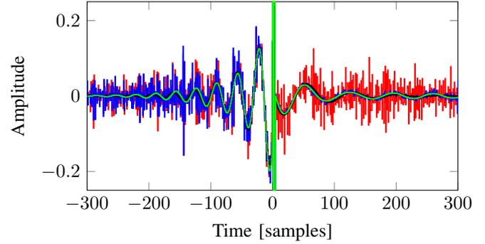
Fig. 4. Estimates  $\hat{\theta}$  from single realization: the non-regularized estimate (—) indicates high variance, whereas using the developed *non-causal* kernel (—) significantly improves accuracy w.r.t. the true impulse response of  $P^{-1}$  (—). Using a pre-existing *causal* kernel (—), only the causal terms ( $t \geq 0$ ) are regularized.
