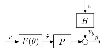
Fig. 1. Inverse-model based feedforward: high tracking performance ( $y \approx r$ ) requires inverse model  $F = P^{-1}$ .
