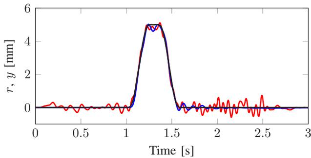
Fig. 6. Results case II (Arizona printer): tracking performance with  $F(\hat{\theta})$  implemented. Without regularization (—), significant errors remain due to high variance of the estimates. The developed regularized approach leads to considerably improved tracking (—) of reference signal  $r$  (—).
