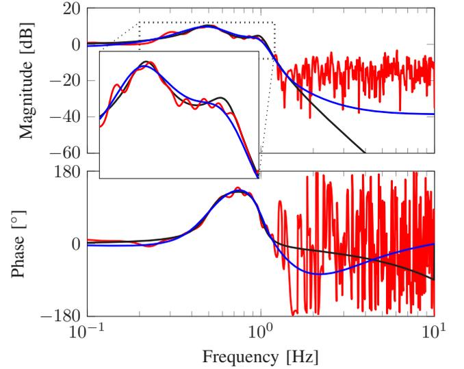
Fig. 5. Results case I: Bode diagram of true inverse system  $T^{-1}$  (—),  $F(\hat{\theta}_{LS})$  (—) and  $F(\hat{\theta}_{ReLS})$  (—). The decreased variance of  $\hat{\theta}_{ReLS}$  results in a smoother frequency response, also at high frequencies where the signal-to-noise ratio is extremely low (approximately  $-23$  dB at 2 Hz).
