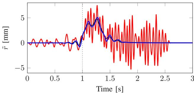
Fig. 7. Results case II (Arizona printer): feedforward signals  $\tilde{r} = F(\hat{\theta})r$ . Using regularization (—) leads to smooth feedforward signal that closely matches the optimal feedforward  $T^{-1}r$  (—). Without regularization (—), the high variance of the estimates leads to erratic control actions. To compensate for the NMP dynamics of  $T$ , non-causal control is used: feedforward is applied before the motion task starts at  $t = 1$  s.
