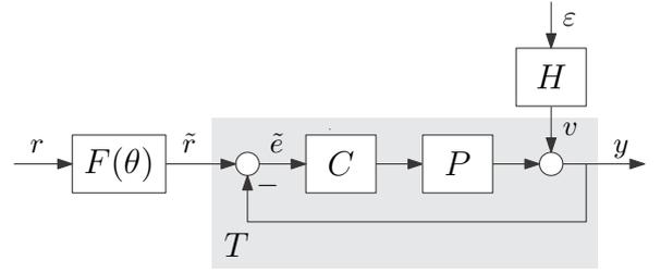
Fig. 1. Closed-loop control configuration with serial feedforward.
