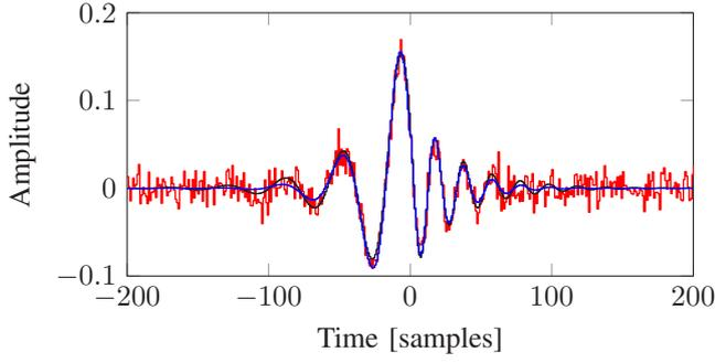
Fig. 4. Results case I: estimated impulse responses. The estimates  $\hat{\theta}_{LS}$  without regularization (—) exhibit high variance. Using regularization (—), the MSE  $\|\hat{\theta}_{ReLS} - \theta^o\|_2^2$  is significantly reduced: variance is traded for some bias with respect to true impulse response (—).
