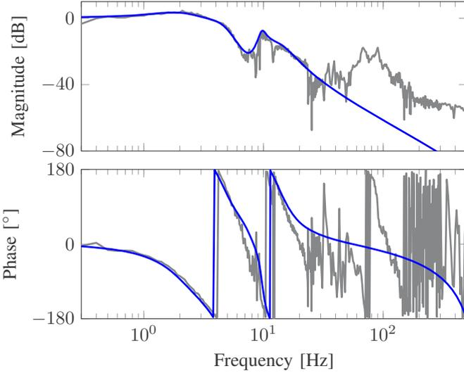
(b) Bode diagram of FRF measurement (—) and model (—) of  $T$ .
