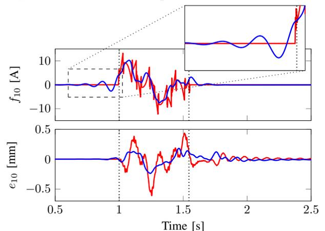
**Figure 3:** Experimental results: non-causal ROBFs (—) enable infinitely long pre-actuation and post-actuation. Compared to (non-causal) FIR basis functions (—), which enable only a small and finite amount of preview, the error  $e_{10}$  is significantly reduced.
