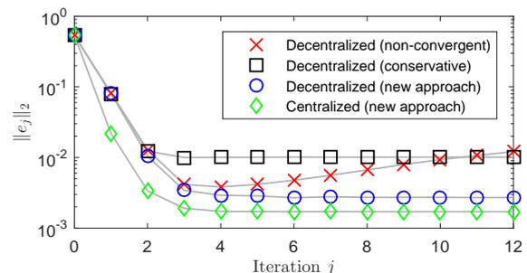
**Figure 3:** The importance of multivariable ILC design: i) ignoring interaction can lead to non-convergent schemes (X); ii) appropriately accounting for interaction can improve performance (O vs. □); and iii) centralized ILC (◇) yields the highest performance at the cost of increased modeling requirements.
