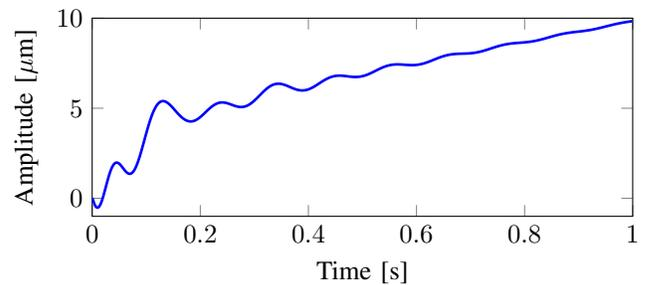
Fig. 3. Impulse response of model  $\hat{P}$ : due to its non-minimum phase dynamics, the system initially moves in negative direction.
