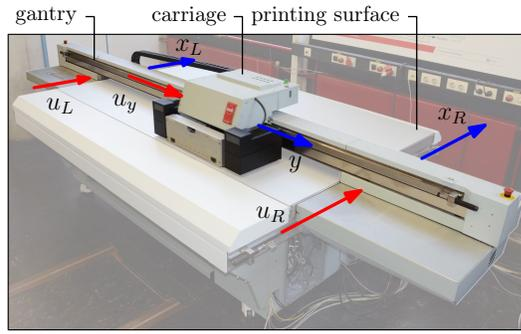
Fig. 1. Océ Arizona 550 GT flatbed printing system, with inputs indicated in red and outputs in blue. For experiments, the system  $P$  between non-collocated input  $u_L$  and output  $x_R$  is considered, which has NMP dynamics.
