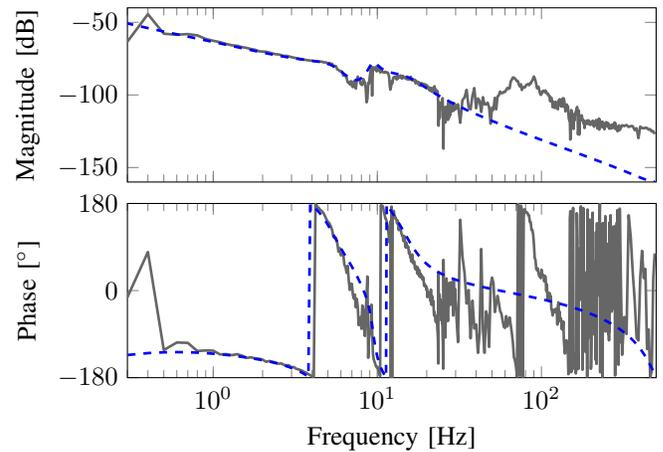
Fig. 2. Bode diagram of FRF measurement of  $P$  (—), and approximate model  $\hat{P}$  (- -). The non-minimum phase dynamics can be observed through the anti-resonance around 7 Hz: the phase lag increases by 180 degrees.
