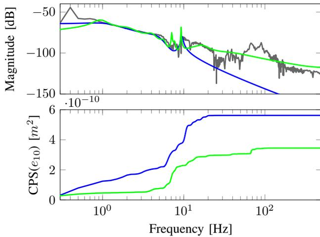
Fig. 9. Experimental results: benefits of cyclically repeating the poles. Bode magnitude diagram of  $P$  and  $F^{-1}(\theta_{10})$  (top) and sample normalized cumulative power spectrum of  $e_{10}$  (bottom). By repeating the poles once (—) compared to the initial pole sets (8) and (9) (—), the power of  $e_{10}$  is reduced at frequencies where  $r$  has dominant power.
