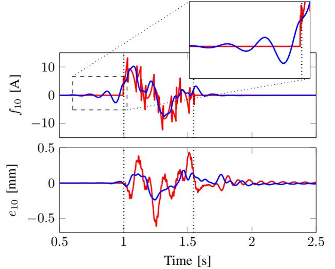
Fig. 8. Experimental results: the non-causal rational basis functions ( $\text{---}$ ) with poles in  $\mathbb{D}$  and  $\mathbb{E}$  enable infinitely long pre-actuation and post-actuation. Compared to the (non-causal) FIR basis functions ( $\text{---}$ ), which enable only a small and finite amount of preview, the error  $e_{10}$  is significantly reduced. The vertical dotted lines indicate the start and end of the motion task.
