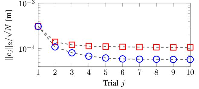
Fig. 7. Experimental results: feedforward learning using ILC. After 10 trials, 45% increased tracking performance is achieved using non-causal rational basis functions ( $\circ$ ) compared to FIR basis functions ( $\square$ ).
