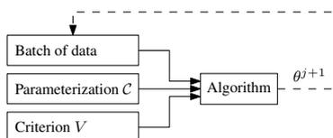
**Figure 2:** Batch-to-batch feedforward tuning from a system identification perspective. Based on a batch of data, parameterization  $C$  and criterion  $V$ ,  $\theta_{j+1}$  is determined and implemented to obtain a new batch of data.
