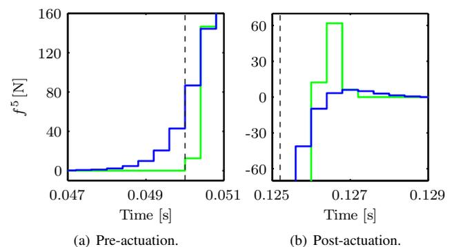
**Figure 3:** The rational parameterization (—) enables pre- and post-actuation of the system, in contrast to the polynomial parameterization (—). The start and end times of the motion task are indicated by black dashed lines.
