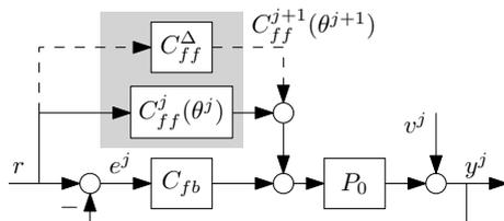
**Figure 1:** Control configuration for iterative feedforward control.
