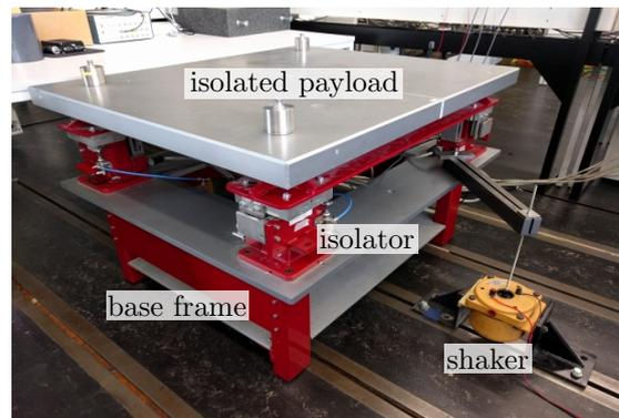
Figure 1: Industrial active vibration isolation system.
