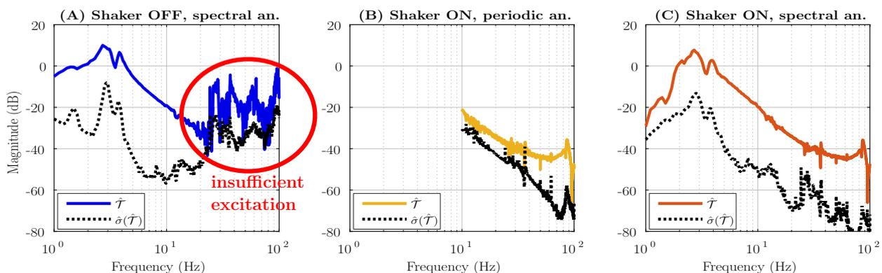
Figure 2: Bode magnitude plots showing the estimated transmissibilities  $\hat{\mathcal{T}}$  and corresponding standard deviations  $\hat{\sigma}(\hat{\mathcal{T}})$  using either spectral analysis or periodic analysis [2].
