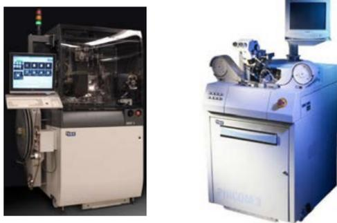
Figure 1: Bonding systems: Die- and Wire-bonder.
