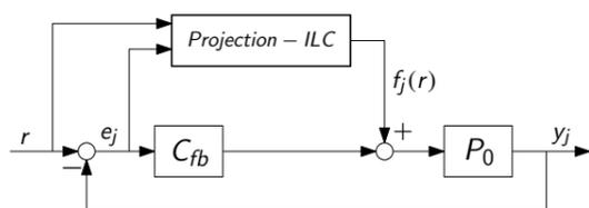
Figure 2: Projection-ILC block scheme.
