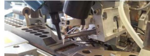
Figure 3: Z-axis of wire bonder.
