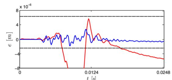
Figure 5: Error time plot after the change in the reference trajectory for S-ILC (red) and P-ILC (blue).
