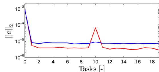
Figure 4: 2-norm of servo error for Standard ILC (red) and Projection-ILC (blue).
